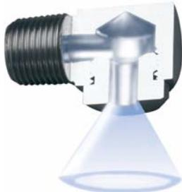
A hollow cone spray pattern consists of droplets concentrated onto the outer surface of a conical shape volume, with no droplets contained in the inside of the conical jet shape. These nozzles are normally used for smoke washing or gas cooling applications in several industrial processes.
